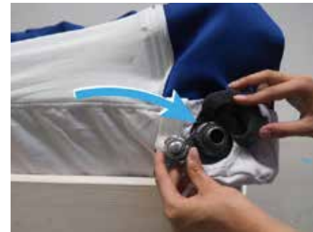
Photo 18: Open front valve cap.
